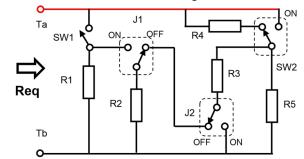
R1 – R5 are all the same value, and in this configuration, you can realize 12 different values, from R/4 to 2R. Here's how you would set the switches to get these resistance values:
