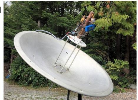
Tilley's home-brew microwave dish used to hear the MRO signal.
